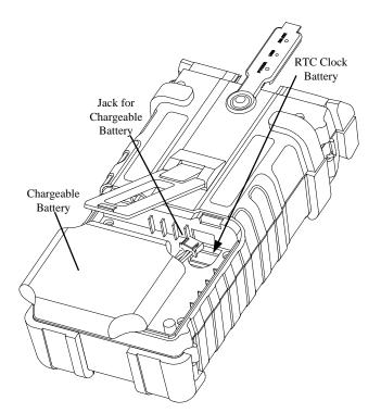
Figure 6-1. Replacing Battery
