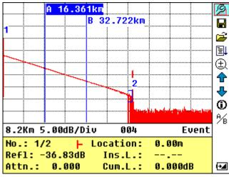
Figure 4-4. Trace Measurement of palmOTDR
