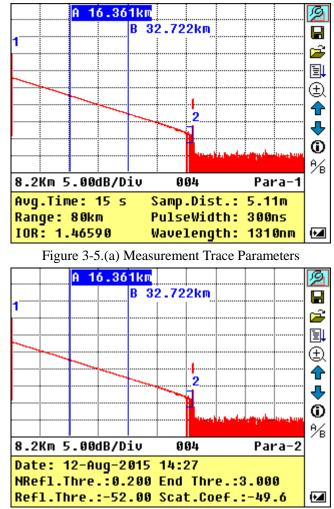
Figure 3-5.(b) Analysis Trace Parameters
