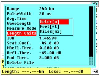
Figure 3-15. Length Units Configuration
