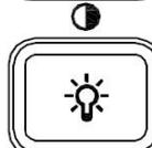
Turn backlight on/off; Long press to adjust contrast
