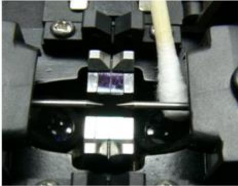
NOTE: Do not touch or hit electrode tips (in this case electrodes do not remove from the splicer).
