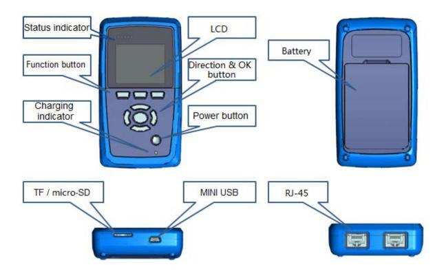
NCT-500 has two RJ-45 ports on the top and has one Micro SD card connector, one Mini USB connector on the bottom. Front have six LED status indicator and one charging indicator.
