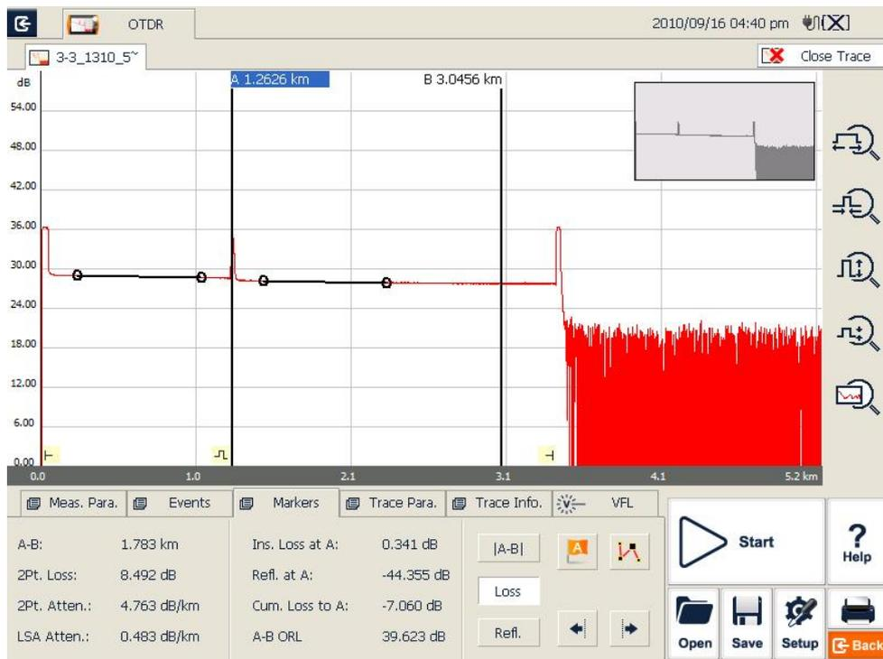
Fig. 12.4 Measure insertion loss in 5-point method
