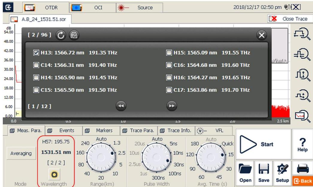
Fig. 9.8b Laser wavelength configuration (DWDM OTDR)
