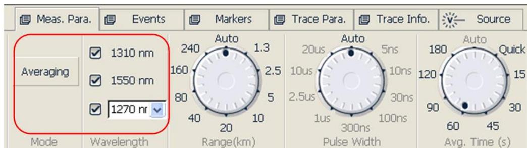
Fig. 9.8a Laser wavelength configuration (Regular and CWDM OTDR)
