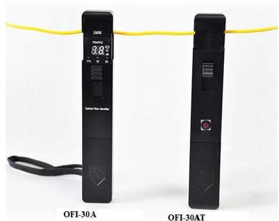
OFI-30A/AT can detect optical signal presence, type and direction anywhere on fibers during optical network deployment, maintenance and troubleshooting. With non-destructive macro-bend detection technology, it introduces no damage to tested fiber or interference to the service on fiber.
