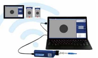
EasyGetWiFi has a USB Type C port to recharge the removable battery. It can work with re-chargers for smartphone, laptop and tablet. USB port of computer and portable battery can also be used to charge the visual inspector. The battery duration is up to 5 hours. The battery can be recharged on-line or individually.
